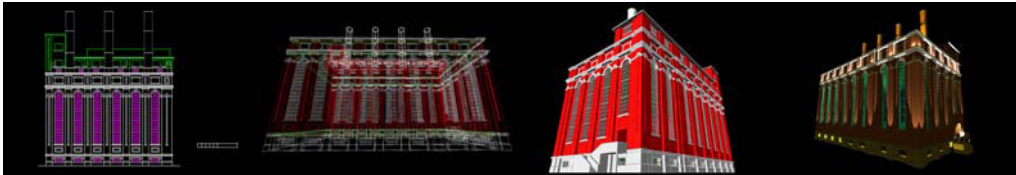
Figure 2 CAD I: Geometric Modeling and visualization. Central Tejo, Lisboa (Eduardo Costa, 2001/02): from the 2d to the photorealistic model
